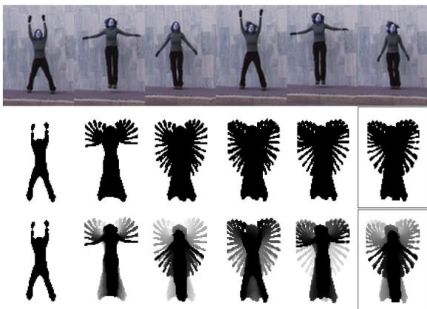
Figure 4: Top: A jumping sequence. Middle: The MEI template Bobick and Davis (2001). Bottom: The MHI template Bobick and Davis (2001). The MEI captures where the motion happens while the MHI template shows how the motion image is moving. The templates at the end of the action, shown in the rightmost column are used for representations.
