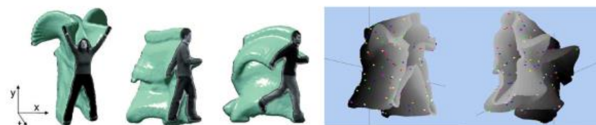
Figure 5: Left: The spatiotemporal volumes used by Blank et al. (2005) to describe the evolution of an action. The 3D representation is converted to a 2D map by computing the average time taken by a point to reach the boundary. Right: The spatiotemporal surfaces of Yilmaz and Shah (2005) for a tennis serve and a walking sequence. The surface geometry (e.g., peaks, valleys) is used to characterize the action.
